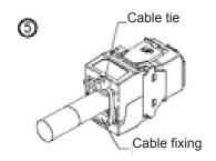
Cable fixing via cable ties.
