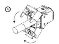
The hinged part of the housing with an suitable crimping tool pressing until its really snapped into place.
