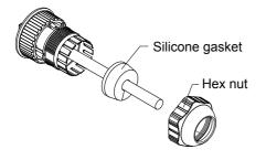
3. Place the silicon gasket and screw on the Hex Nut tightly to ensure the watertight function. Using a hex wrench to help when necessary.
