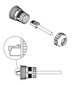
1. Finish the installation of RJ45 Patch cable first and insert it through the IP68 plug housing.
