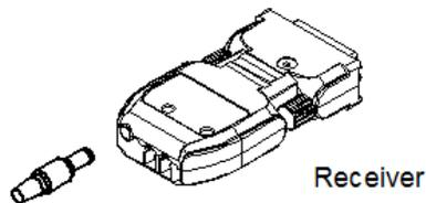
Figure 3 – Connection of power adapter to the receiver
