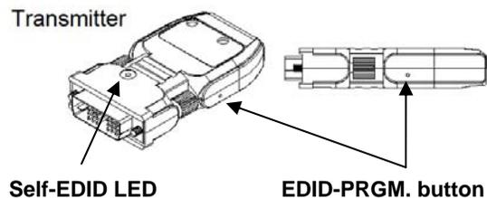
Figure 7 – Position of EDID-PRGM. button and Self-EDID LED
